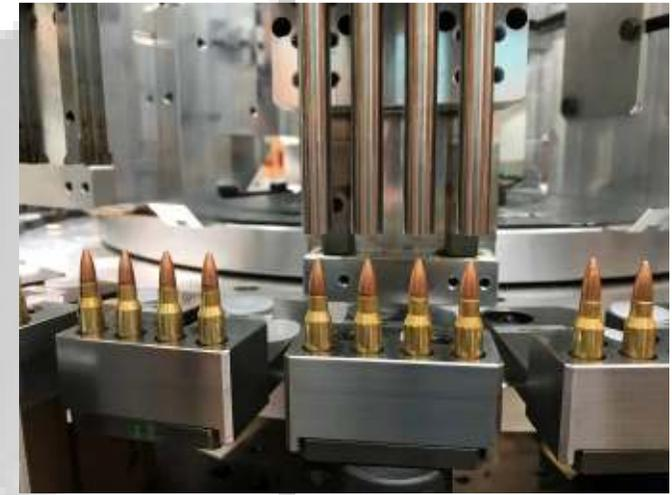
100% Electronic control of the bullet inserting force.
