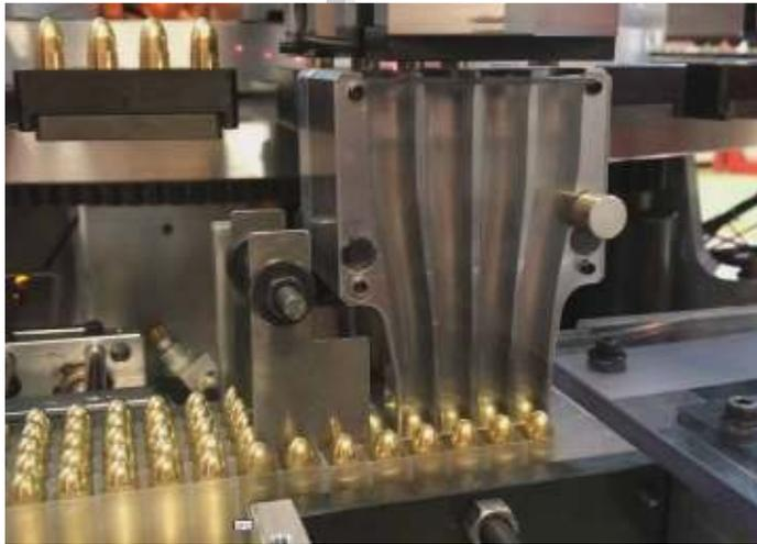
Packing station to fill directly the ammunition tray, full filled tray and empty tray exchanged automatically without any machine stop or production rate decreasing.
