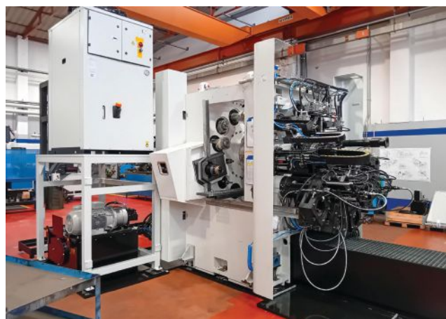
↑ Air-Way's second Buffoli rotary transfer machine, here shown during assembly in Italy, will be delivered early 2025.
