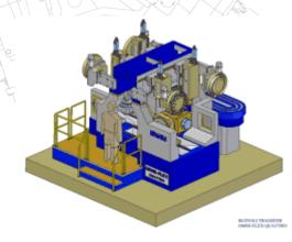
This two-pallet machining center is capable of complete machining on all 6 sides including any angular orientation. The machine is equipped with 2 chucks, each with 2 full CNC rotary positioning axes, 80 tools in 4 magazines of 20 tools each and 4 spindle motors of 25 kw (12,000 rpm), complement its speed and flexibility. Tool change over in less than 30 minutes.
