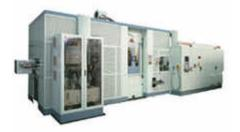
This flexible-universal-expandible version of the CNC bar transfer machine most prevalent globally, is capable of complete machining of both end and transverse part features in one chucking, with the shortest cycle times.
