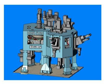
The **OMNI-TURN-TRANSFERS** allow manufacturing of precision parts requiring heavy turning millina operations along with operations, angular or transversal drilling. threading, broaching. marking, assembling, gauging, etc. These patented machines solve the challenges of high productivity of complex components while maintaining the versatility and guick change over capabilities necessary for batch manufacturing.
