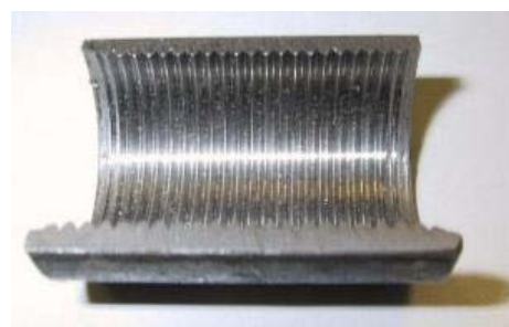
Ø ¾" x 1.7" Conical Thread (Ø 25.8 x 43 mm) Tap life of up to 5,000 parts
